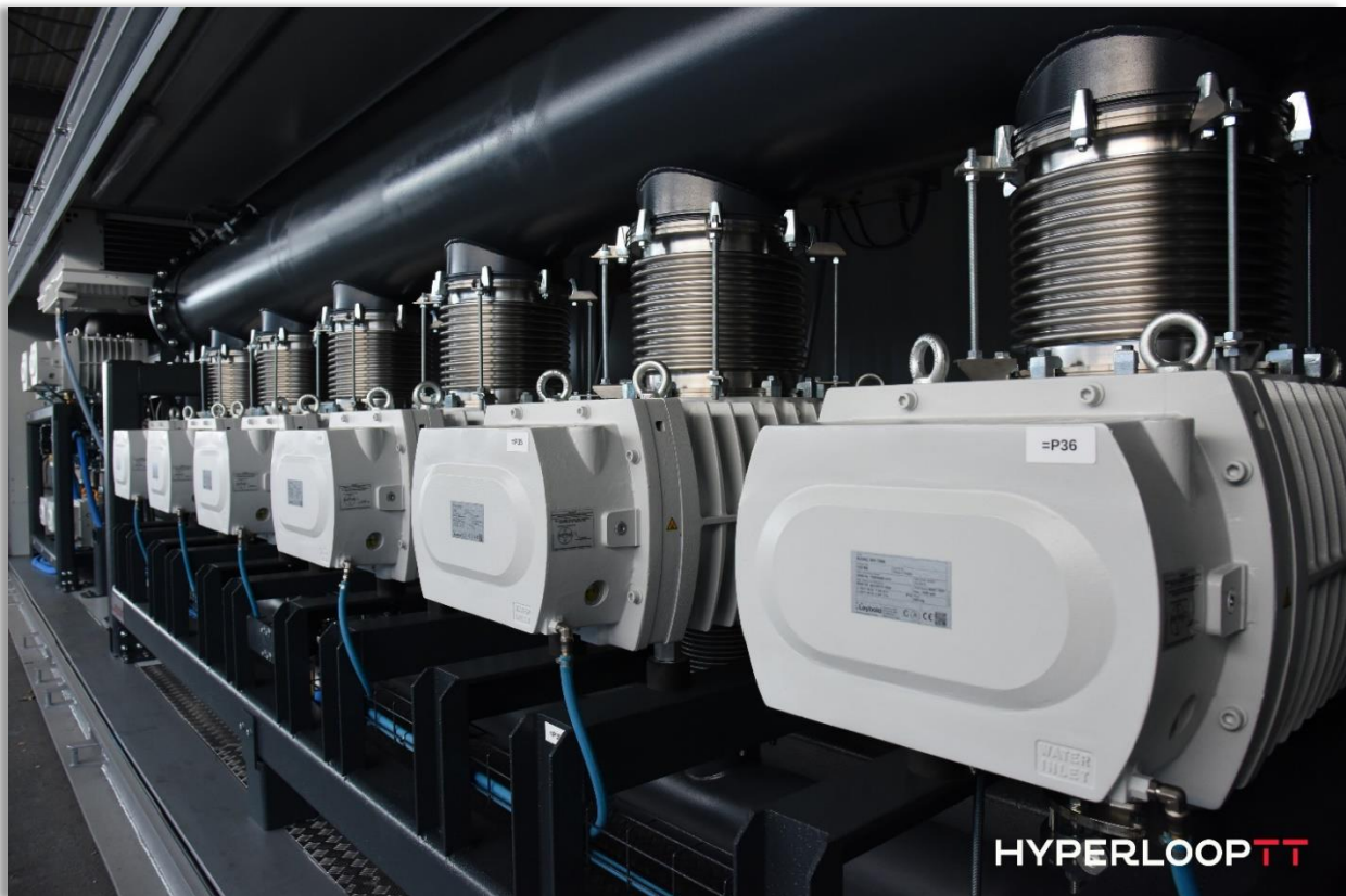
Exhibit 2-8: Vacuum pumps and modular housing, Courtesy of HyperloopTT
