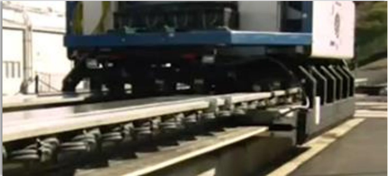
Figure 2-5: Inductrack illustration, Courtesy of HyperloopTT
